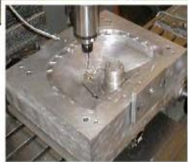
All the Die for investment casting plant are made in- house, on VMC machines to reduce the cost.
